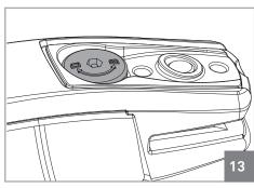
Information engraved on the unlock shaft D=Unlock || B=Lock
