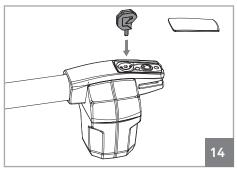
**02** • Insert Release key on the unlock shaft.
