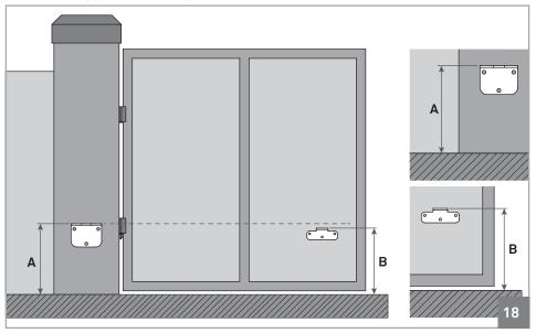
**Dimension A •** *Vertical distance* from the floor to the top of the rear support . **Dimension B •** *Vertical distance* from the floor to the top of the front support.
