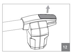
01 • Remove the plastic cap from the rear end
