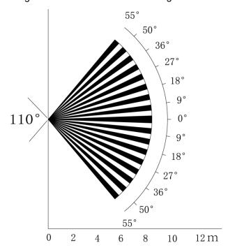
The vertical detection distance of the sensor is 2 m–10 m, 1 m–14 m or 1 m–12 m. Figure 6-2 Vertical detection distance
