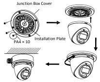
Figure 2-10 Fix the Camera to the Junction Box For Type IV and Type V camera:
