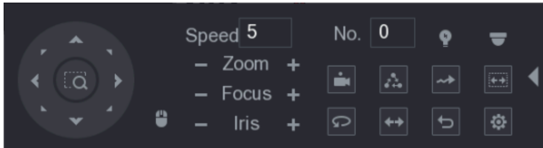
Figure 5-57 Expanded PTZ control panel
