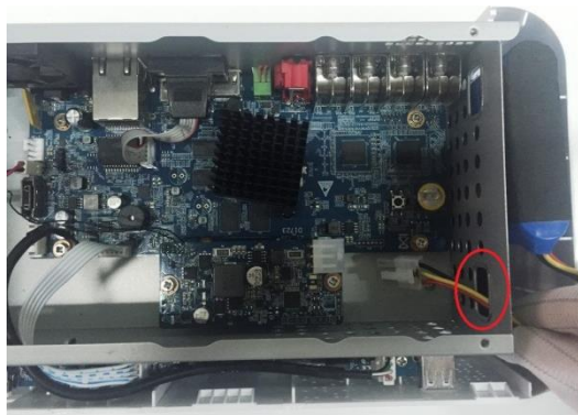
Figure 2-6 Pull battery cable through hole
