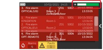
5. The Delay Override Option is now enabled on the main display, allowing the operator to activate the outputs configured for delay in the Cause and Effect I/O Matrix before the countdown is finished.
