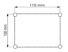
STEP 1 According to the figure, mark the required hole on the wall.
