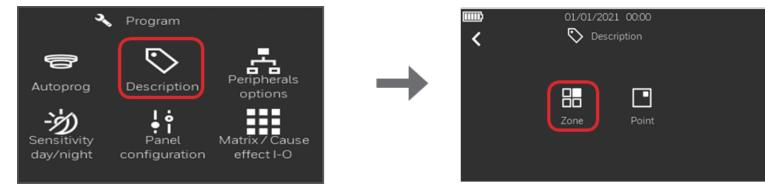
2. To define a Zone, press on the icon  $\mathbb{B}$ , then press at the right side of the zone number (e.g. Z01), below the icon  $\mathbb{S}$  and type the name of the zone. A QWERTY keyboard appears to enter the description. It is possible to insert up to 20 characters. Press the "enter" key to save and confirm the zone description. Press the back arrow  $\mathbb{S}$  to go back to the previous screen.
