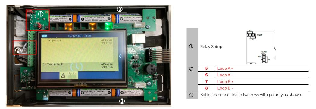
Fig. 16: LT-159 setup and connections overview
