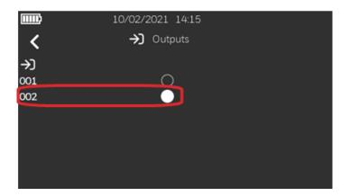
3. To end the Output test, press on the full dot. Press the back arrow to go back to the main screen.
