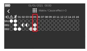
4. When a delay is active, a timeline appears on the main screen to show the delay progresses. If another Zone set to works with the delay goes into alarm, a + mark appears near the delay bar, indicating that another countdown is started.
