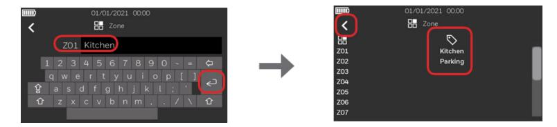
3. To define a Point, press on the icon , then press at the right side of the device number (e.g., S001) below the icon and type the name of the device. It is possible to insert up to 20 characters. Press the "enter" key to save and confirm the zone description. Press the back arrow to go back to the previous screen.
