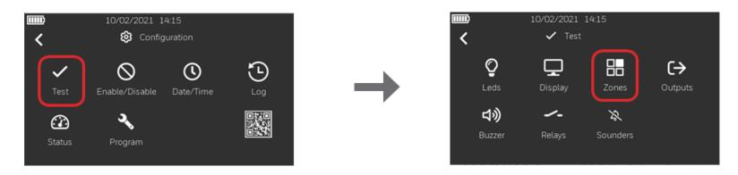
2. Click on the icon 🕐 near the Zone you would like to put in Test. The Test icon 🖍 will be displayed near the selected Zone and label will be updated; in this example ZO2. Press the back arrow for go back to the main screen.
