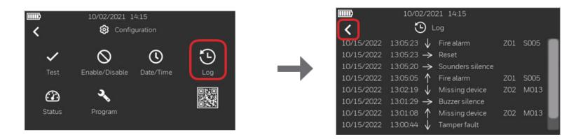
2. The events are shared in sequence, the latest is on top and the oldest is on the bottom of the list. Are shown date and time of the events, the type of the events, the Zone number and the related device address. Are also shown the commands released from the panel.
