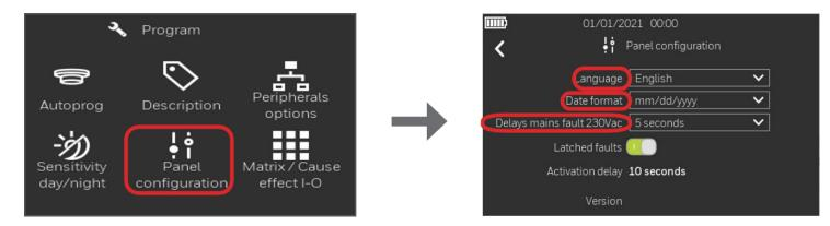
3. Pressing the arrow down on Date Format field, you can change the date format between mm/dd/yyyy, yyyy/mm/dd or dd/mm/yyyy. Data Press on the back arrow to go back.
