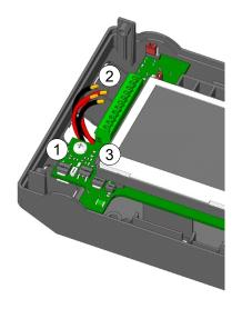
Fig. 14: Cable routing and connections
