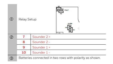
Fig. 15: LT-32 setup and connections overview
