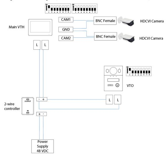
Figure 2-2 Network diagram (with line termination terminal and branch terminal)
