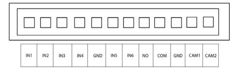
Figure 3-11 RS-485 and power output port
