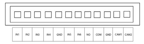
Figure 3-6 RS-485 and power output port
