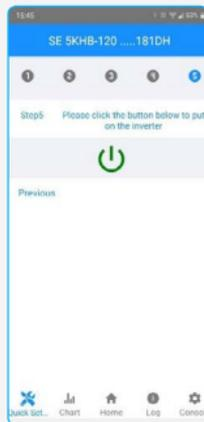
4. When in Quick Setup, DO NOT MAKE ANY MODIFICATIONS. Any modification will alter the remote monitoring of the inverter. On the upper gray ribbon, with buttons from 1 to 5, select the 5 button, the button for ON/OFF will appear. Press the symbol for ON (green) and the inverter will be starting shortly, and the symbol for OFF (red) to power off the inverter.
