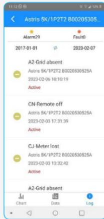
LOG shows all the recorded events that happened during the functioning of the inverter such as: notifications, alarms (non-critical), errors and failures (critical).
