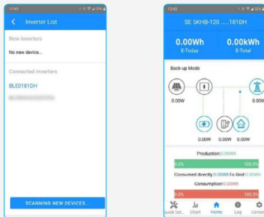
3. Press SCANNING NEW DEVICES. After a few seconds, a new device will appear in the New Inverters section. Press it and it will be transferred into the Connected Devices section. The management option page will open up as shown in the picture below.
