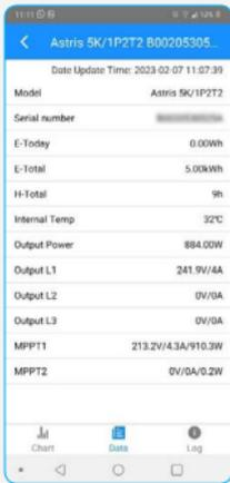
With the DATA button technical data can be obtained about the inverter such as: model, S/N, rated power, temperature, output voltage, PV input voltage etc.
