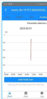
The price per Kilowatt can be observed also, and the savings accumulated during solar energy implementation. In ANALYSIS from the Parameter Selection can be selected different electrical parameters with variables that will be represented on graphs.
