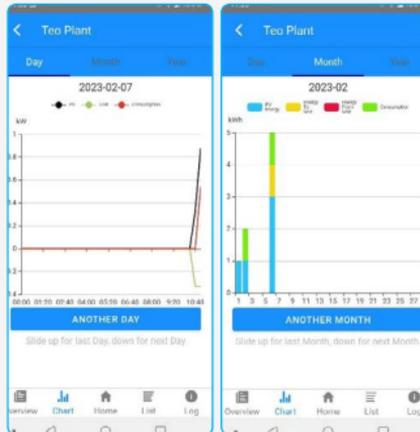
The CHART button displays the graphical representation of the following information: energy production, consumption and sent to the electricity grid on daily, weekly and yearly basis.
