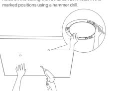
3 Fix the bracket. Option A below applies to most general cases. For ceilings with weak strength (such as plasterboard) and APs provided with plastic nuts, please choose Option B.
