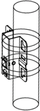
Figure 3-3 Mounting the Plate on a Pole
