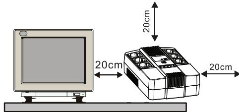
In addition, at least 20cm space should be reserved around the UPS (including the top) to avoid interference with surrounding devices and ensure the heat dissipation.
